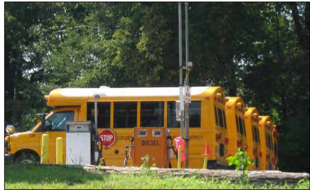
Covering the outdoor fueling station at the bus maintenance facility would decrease the stormwater pollution potential of the fueling activities.
